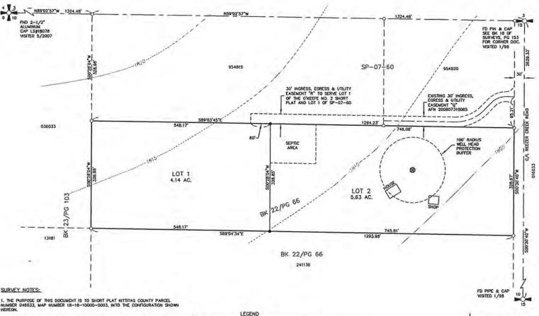
2. THIS SURVEY WAS PERFORMED USING A TRIMBLE SE SERIES TOTAL STATION. THE CONTROLLING MONUMENTS AND PROPERTY COMPRESS SHOWN HEREON WEEK LOCATED, STAKED AND CHECKED FROM A CLOSED FIELD TRAVERSE IN EXCESS OF 1:10,000
